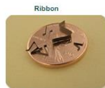
Ribbon Tungsten Ribbon .001 and .003" thickness
